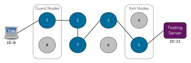
Figure 1: The CS666 Tor network. Note that the lines indicate connections in the Tor circuit, not individual network links.
